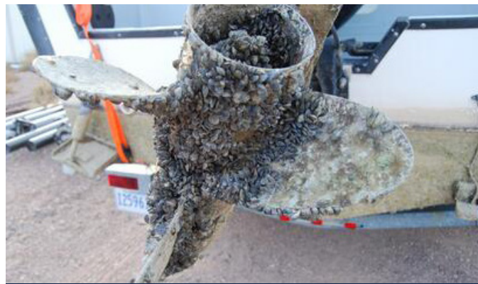
Mussels coat the propeller of an outboard motor. (Photo courtesy of U.S. Fish and Wildlife Service)
